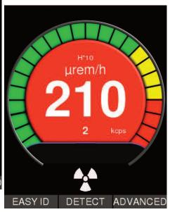
The Detect measuring mode is a tool to locate radiation sources by giving rapid visual and audio feedback to the changing dose rate of incoming radiation. After switching to Detect mode, the user can localize the radiation source by monitoring (in real-time) the auto-scaling chart with color enhanced areas representing the dose rate history of the last few seconds. When the source has been localized, the user may then initiate an "Easy ID" to quickly identify radiating nuclides.
